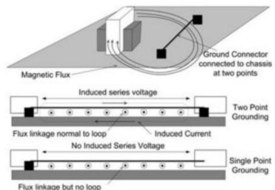
**Figure 2: In an ideal world, all points labeled "ground" are at exactly zero volts. Given a path, electricity will flow. Electricity and magnetism are interrelated, a good thing since motors depend on that relationship to work, but not good when current flow is unwanted. Source: The Circuit Designer's Companion, Peter Wilson.**
