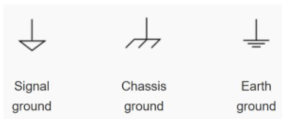
**Figure 1: There are three different electrical symbols for ground, indicating context within a schematic. Source: Wikipedia.**
